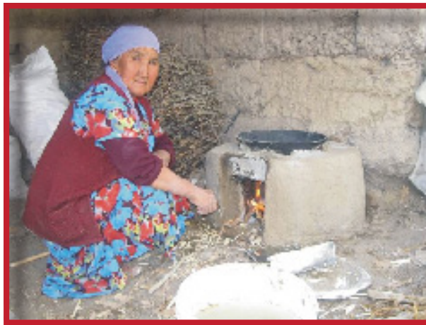
Testing of the energy efficient hearth
